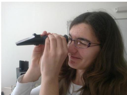
**Image 2:** Measuring sugar with a refractometer
