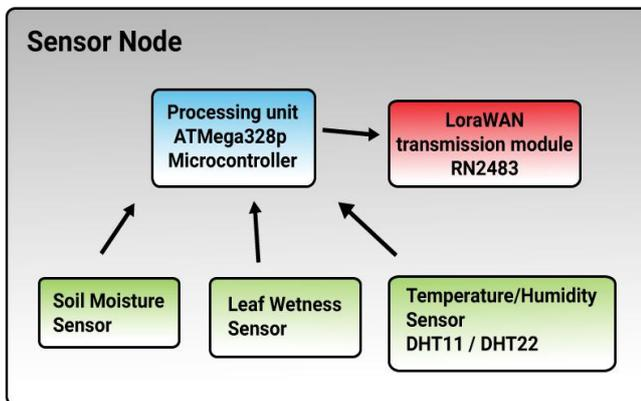
Fig. 3 Sensor node structure diagram for agriculture parameters
