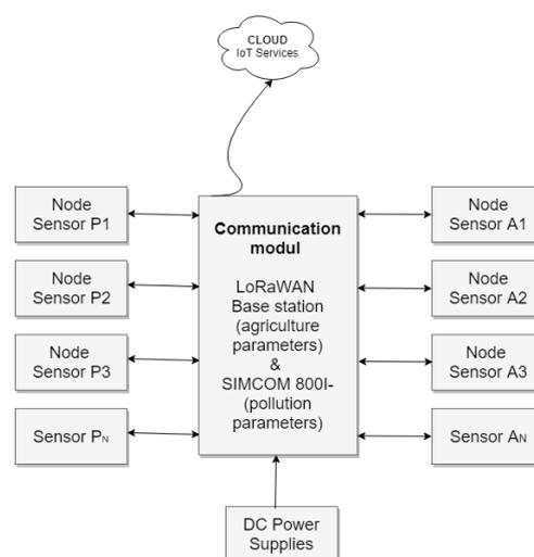
Fig. 1. Wireless sensor network topology diagram
