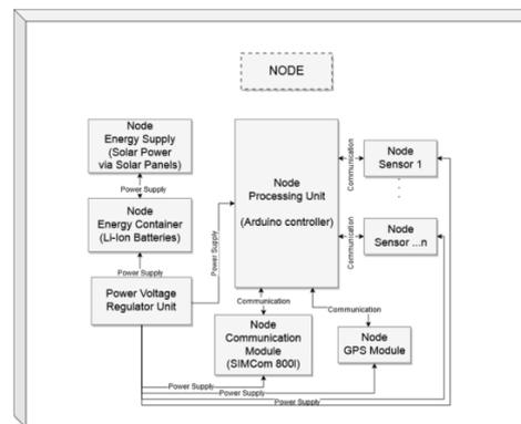
Fig. 4 Sensor node structure diagram for pollution parameters
