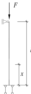
Fig. 1 Static scheme of the investigated column
