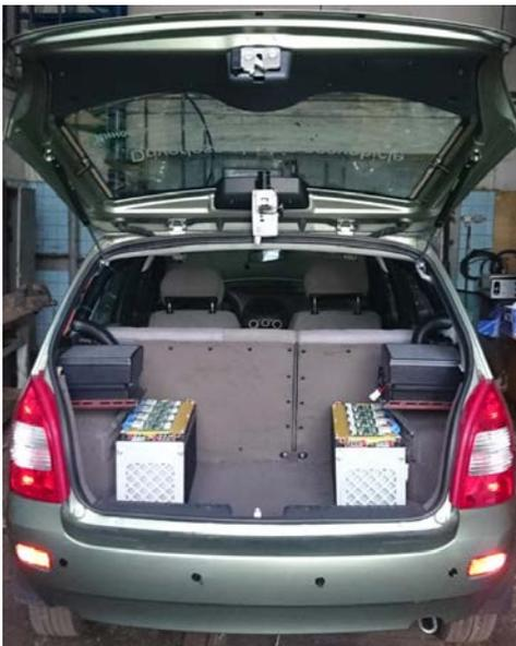
*Fig. 9 Experimental model of a driverless vehicle with the energy storage system*
