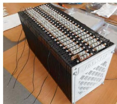
**Fig. 7** The experimental sample storage module of the traction battery
