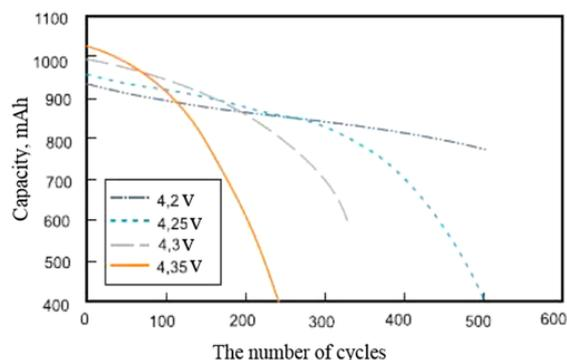
**Fig. 2** The effect of the charging voltage at the battery service life
