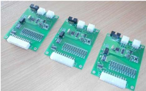
*Fig. 8 Balancing boards*
