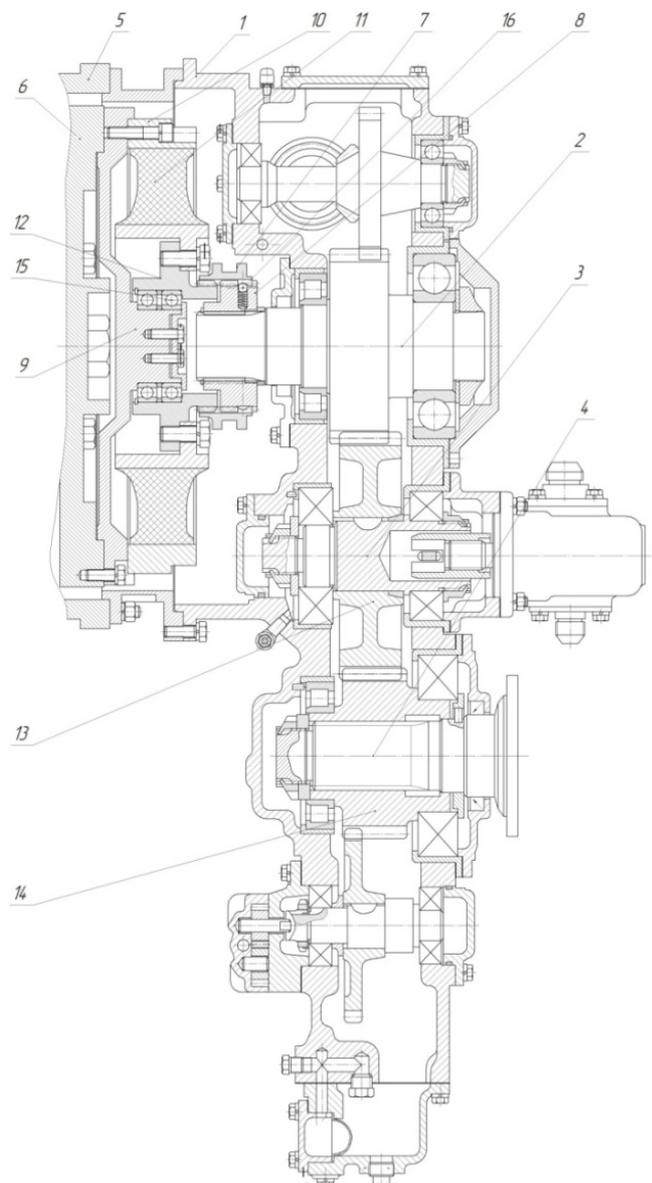
Fig. 7. Modernized design of matching reduction gearbox.
