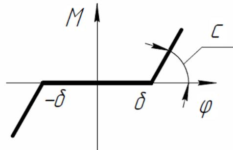
Fig. 3. Schematization of nonlinear function with dependence of the moment on the angular coordinate (nonlinearity with a dead band without saturation).
