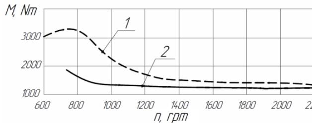
**Fig. 8.** Amplitude and reverse characteristics of the dynamic torque in the pre-torque-converter zone of the HMT: 1 – original (serial produced) version of a matching reduction gearbox; 2 – the developed sample of a matching reduction gearbox.
