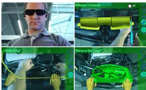
Fig. 3 Visual instruction manual for vehicles maintenance in BMW (source: BMW AG).
