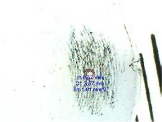
Fig. 6 Example trace of wear on the flat surface, r_o=0,258 mm, S=0,209 mm 2 .
