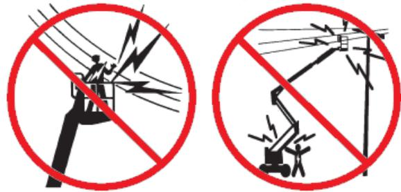
Fig. 11 Prohibition on nearing power lines [6]
