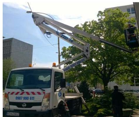
**Fig. 5** Articulated – telescoping platform lift on an automobile chassis
