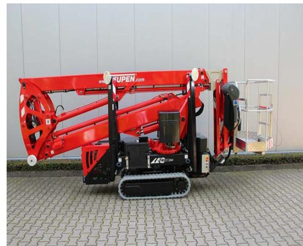
**Fig. 6** Platform on its own belted chassis [3]
