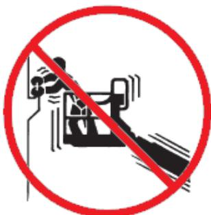
Fig. 14 Prohibition on pulling/pushing objects outside the platform [6]
