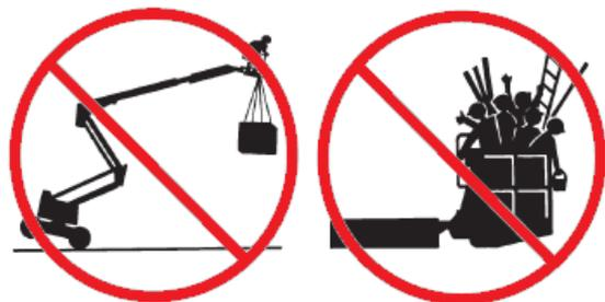
Fig. 15 Prohibition of lifting loads and prohibition on overloading of a platform [6]
