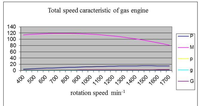
Fig. 3 Total speed characteristics of gas engine depending on rotation speed (test engine)
