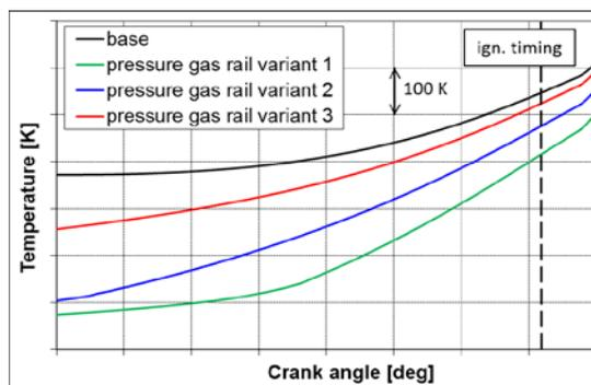
Fig. 7 Scavenging with a stoichiometric mixture: temperature in the pre-chamber at different gas rail pressures.
