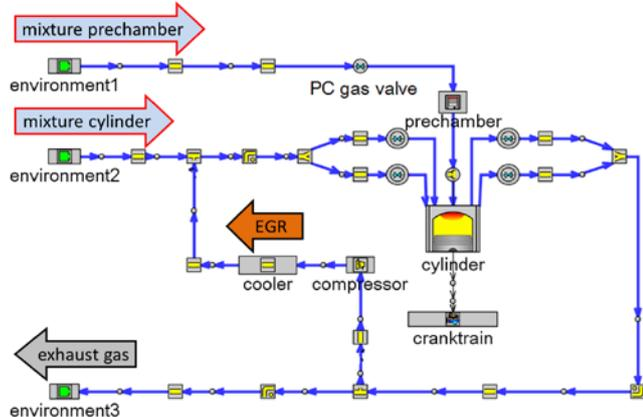
Fig. 3 Topology of the 1D model of the single cylinder research engine including the EGR system.
