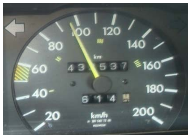
Figure 3. The vehicle speed which corresponding speed of drive pinion gear for rear axle assembly at 3000 rpm
