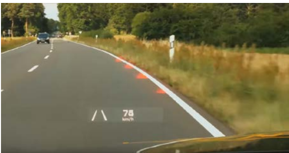
Fig. 2 Driver Assistance System for lane keeping
