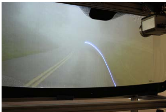
Fig. 3 Driver Assistance System for lane keeping
