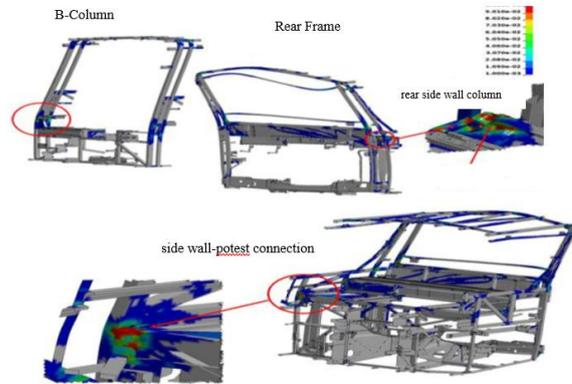
Fig. 6 Structure deformations.
