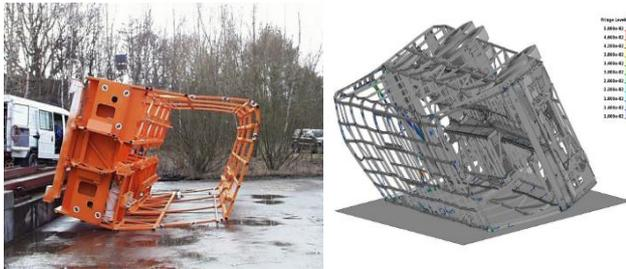
Fig. 2 Rollover test of a passenger bus.
