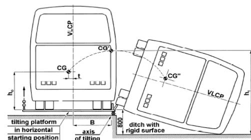
Fig. 1 The centre of gravity positions for rollover test in ECE R66 [4].
