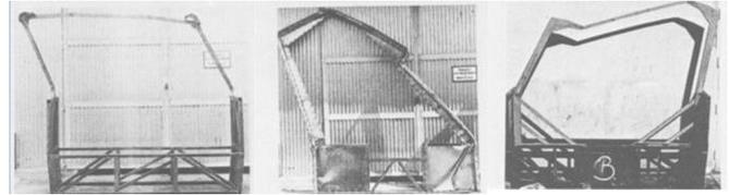
Fig. 5 Different profiles of structures after rollover.
