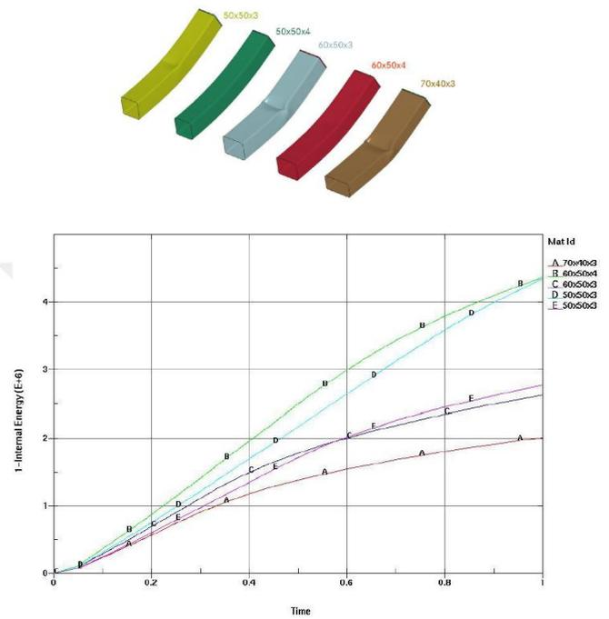
Fig. 9 Deformation behaviors under load of pipes in different sections. Examination of an intercity vehicle, it was observed that the first overturn test was not able to pass the test and reinforcement measures were investigated (Figure 10).
