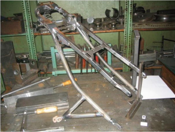
Fig. 4 First prototype BMW K71 rear frame.
