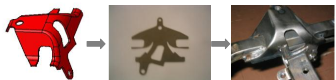
Fig. 3 Process of prototyping the complex element.
