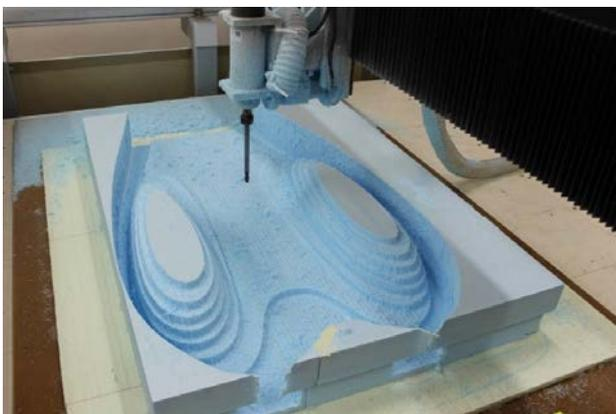
Fig.6 Rough milling of one model part
