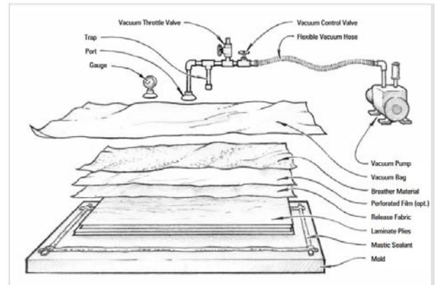
**Fig.11** Typical components of a Vacuum Bag Molding Process
