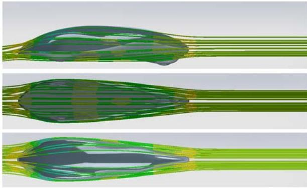
Fig.4 Airflow of the vehicle - side view, lower part, top view
