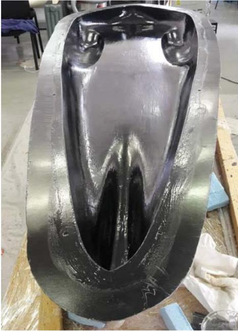
**Fig.8** Interconnecting resin HAVEL 97
