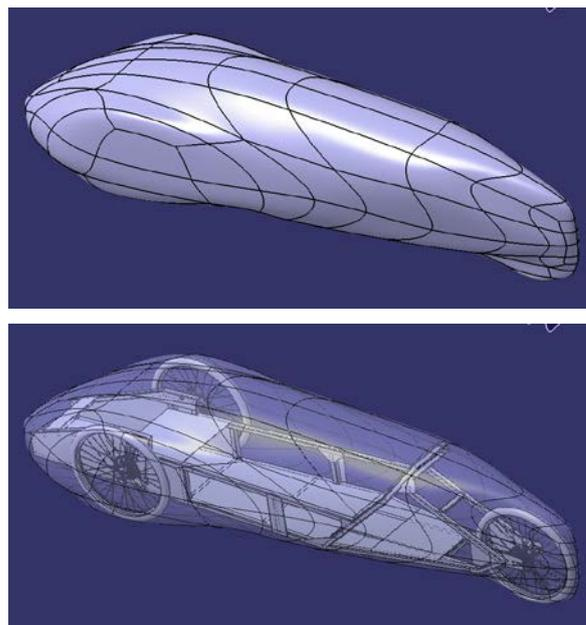
Fig.2 CAD design of body vehicle a) the vehicle bonnet, b) the vehicle internal support frame
