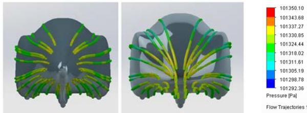
Fig.5 Airflow - view of the rear and front part of vehicle; scale of pressure
