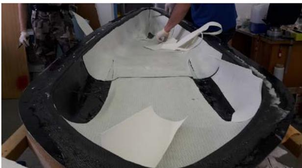
**Fig.10** Fourth layer Coremat XM
