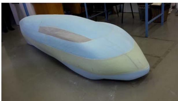
Fig.7 Experimental vehicle - milled model
