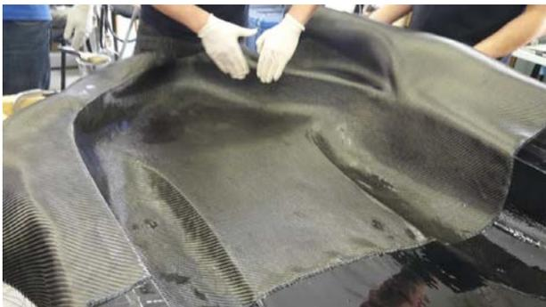
**Fig.9** Deposition of carbon fabric into front part of the mold
