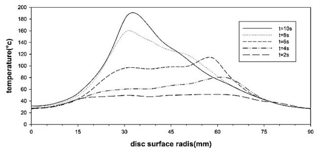
Fig. 10 Temperature diagram over the surface path-1 at t=2,4,6,8,10s
