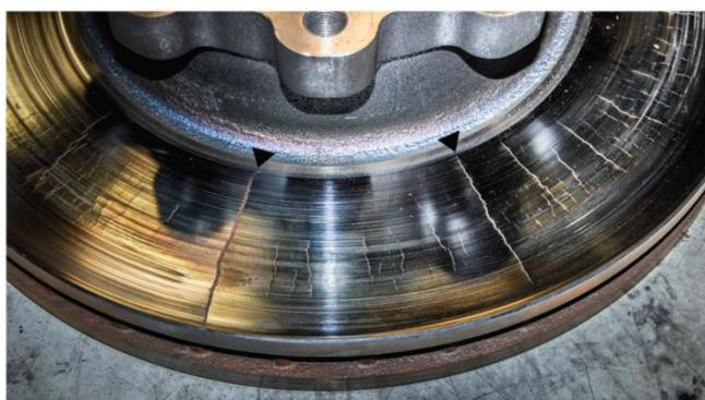
Fig. 1 Radial thermal cracks due to hard braking in heavy vehicles<sup>1</sup>.
