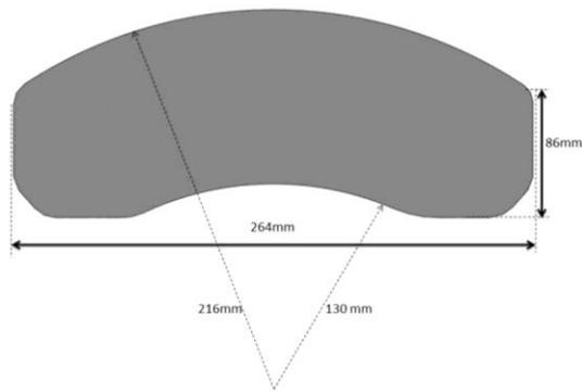
Fig. 3 Brake pad geometries
