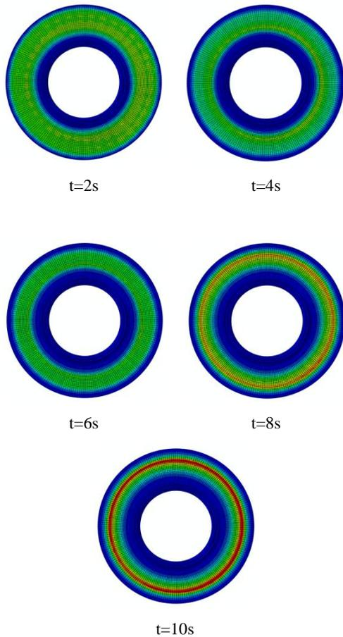
Fig. 11 Schematics of hot bands formation by passing the time (hot bands are depicted in red)
