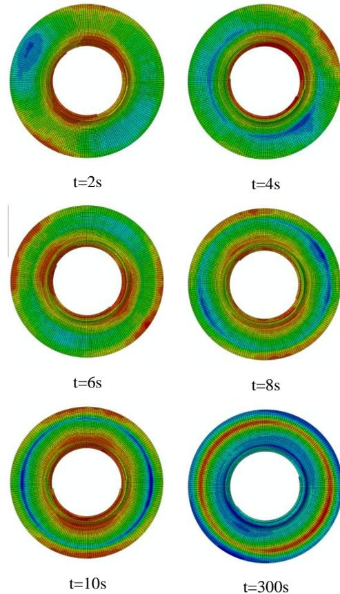
Fig. 13 Circumferential stresses for brake disc surface at t=2, 4, 6, 8, 10, 300s
