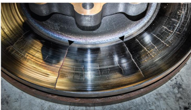
Fig. 1 Radial thermal cracks due to hard braking in heavy vehicles 1 .
