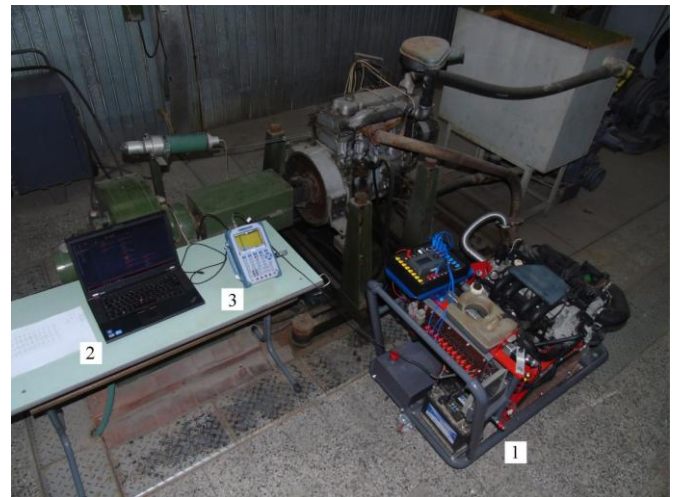
Fig.2. Overview of the test bench SKAD-1: 1-test bench; 2- computer equipment; 3-measuring equipment
