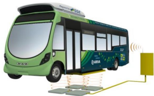
Fig. 2 Wireless charging of electric buses [12].
