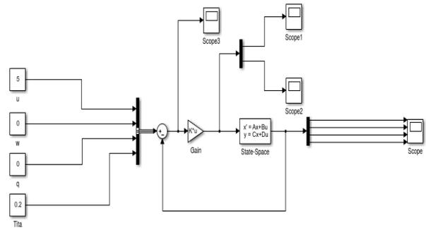
Fig. 8 Closedloop system with LQR compensator matrix K.
