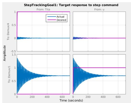
Fig. 10 Reaction system to a step function in the control chanel.
