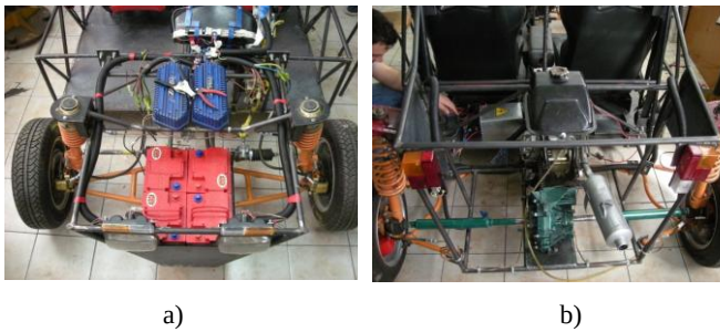
Fig. 2 Front axle with in-wheel electric motors and batteries (a) and Rear axle with the conventional passenger-car final drive, driven by IC engine (b) [1]
