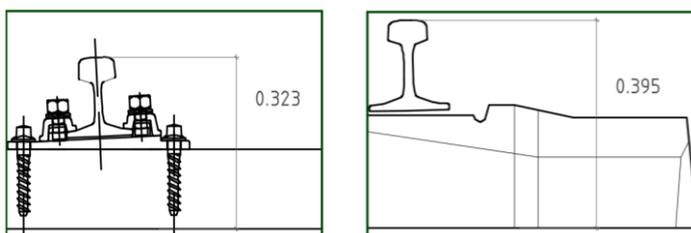
Fig. 1 Rail track fastening ПІАК 68II and SKL14
