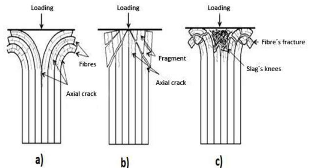
Fig. 3 The types of material damages: - a) The fibres disruption b) Fragmentation c) Brittle fracture [5].
