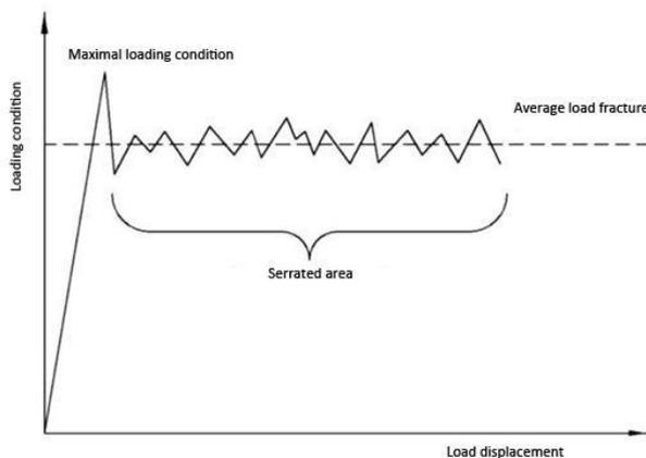
Fig. 2 Graph of the impact energy absorbing [5].
