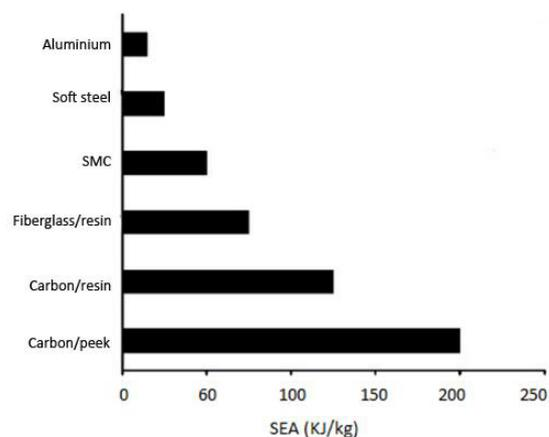
Fig. 4 The energy absorption of specific materials [3].
