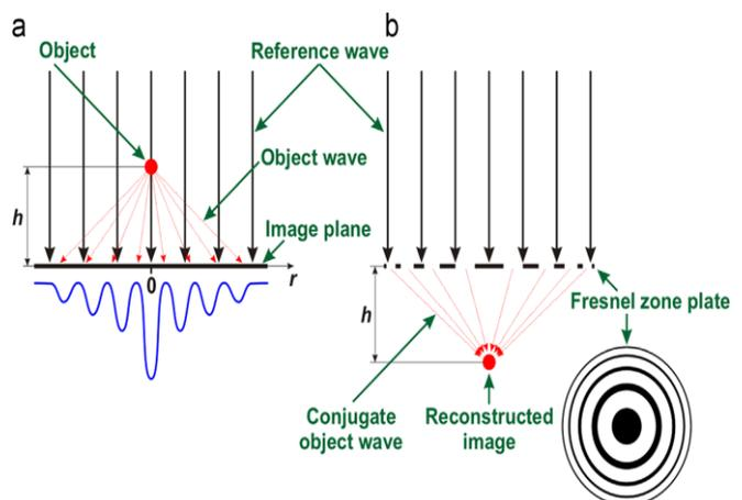
Fig. 1: Optical hologram recording (a) and reconstruction (b) [10]
