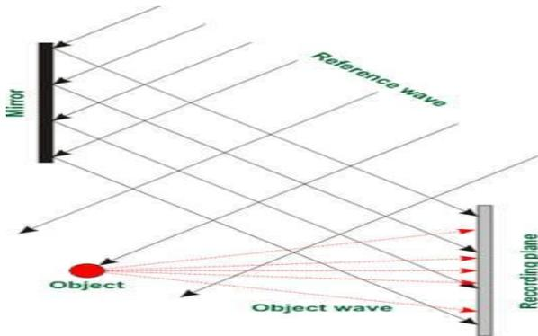
Fig. 2: Optical hologram with inclined light beam [9]
