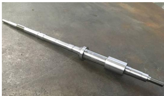
Fig. 4.2 - Shaft of the test bench
