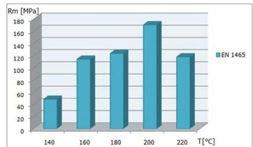
Figure 5. Comparison of the joint strength of the STN EN 1465 test depending on the curing temperature of the adhesive
