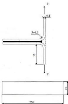
Figure 3. Sample shape for strength test according to EN ISO 11339
