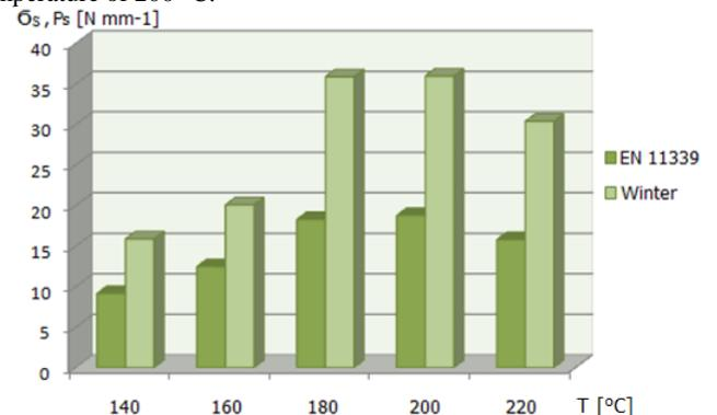
Figure 6. Comparison of the initial joint strength of tests according to Winter and ISO 11339 depending on the curing temperature of the adhesive
