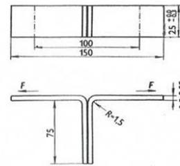
Figure 4. Sample shape for Winter peel strength test
