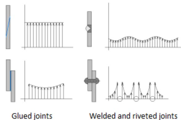
Figure 1. Stress profile in connections [5]
