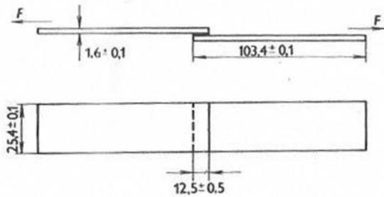
Figure 2. Sample shape for shear strength test according to ISO 4587
