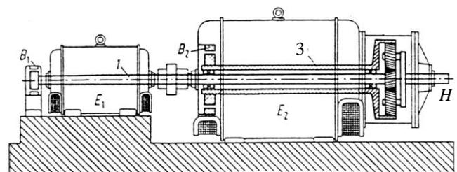
Fig. 3. Twin-motor two-speed drive with an  $\overline{AI}$ -PGT operating as summation differential [3]
