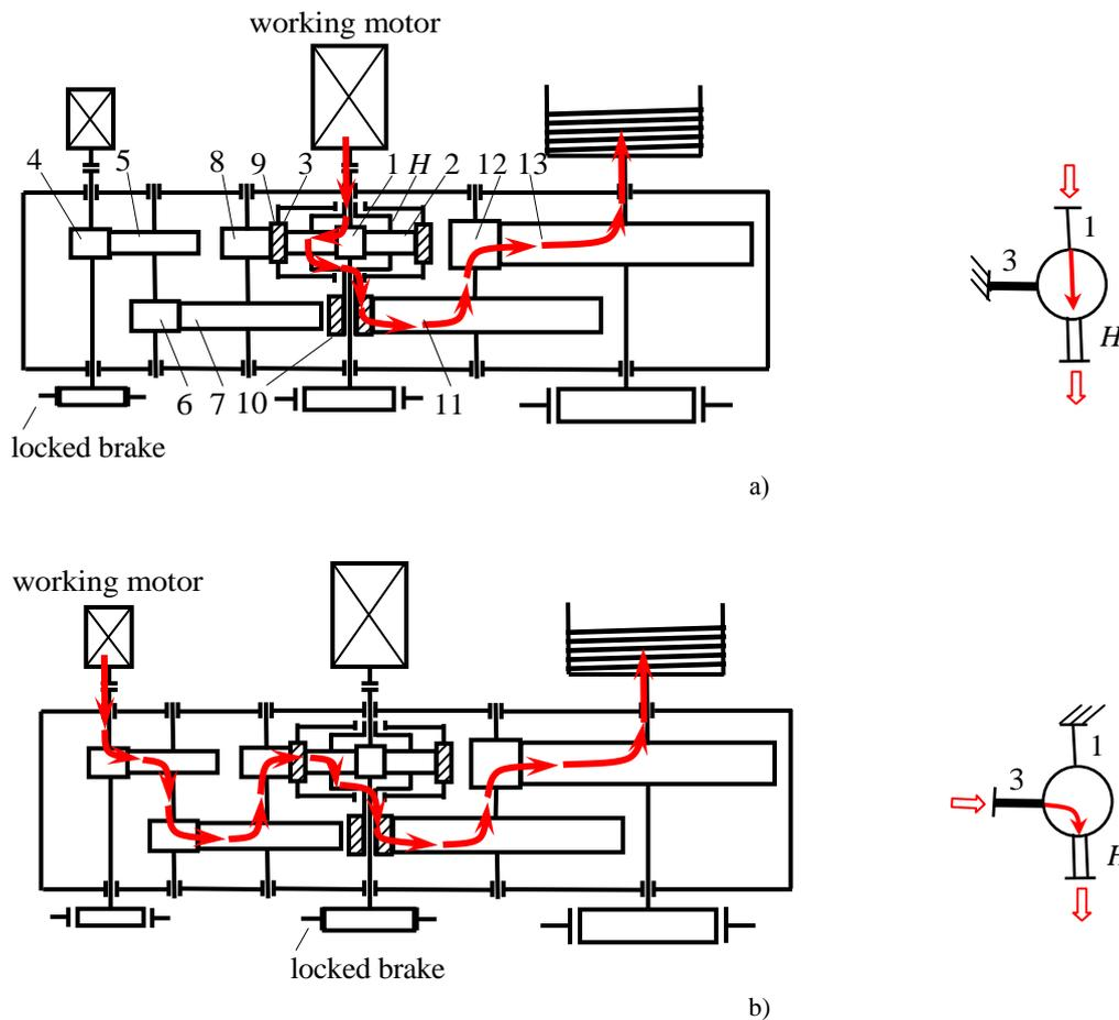
Fig. 5. Operation of AI-PGT as a stage of a two-speed gearbox of a hoisting mechanism [3, 5]
