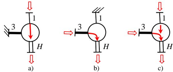
Fig. 4. Working modes of the PGT from figure 3
