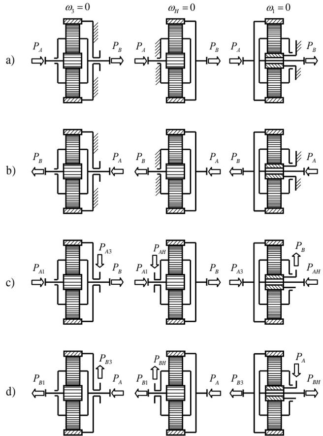
Fig. 2. Working modes of  $\overline{AI}$ -planetary gear train [3, 4]:
