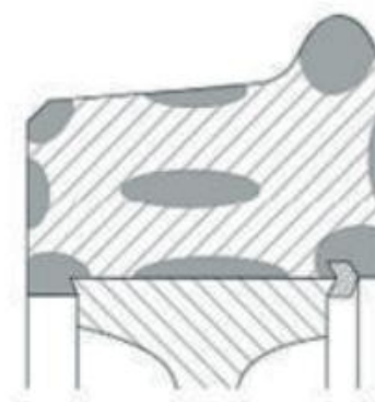
Fig. 1. Places of fatigue destruction of bandages that can serve as the beginning of fatigue wear are highlighted.
