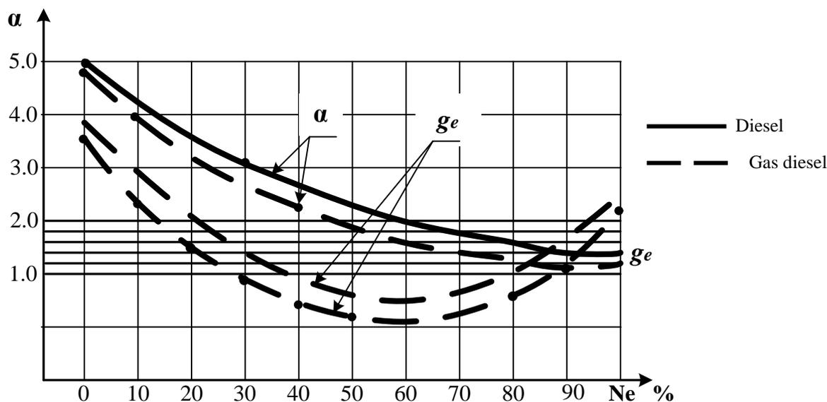
Fig. 1. Variability the parameters of diesel and gas diesel
