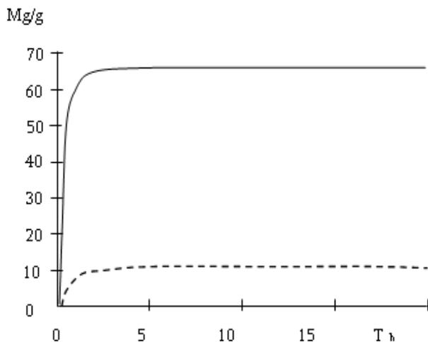
Fig. 1. The adsorption rate of  $CH_4$  on zeolites.
