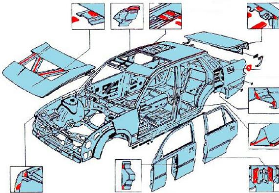
Fig. 2 Glued joints of the car body [6].
