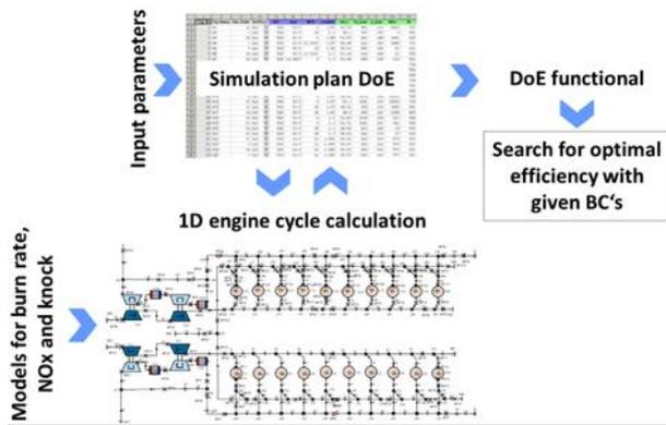
Fig. 4 Procedure for applying DoE methods for 1D simulation.
