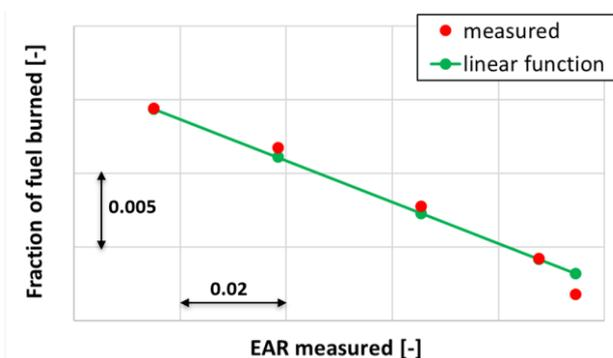
Fig. 2 SCE measurement: Fraction of fuel burned as a function of EAR.
