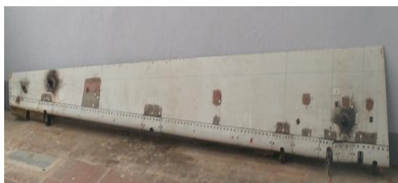
Fig.1. The elevating ruder after lightning strikes impact by the end of crushing tests.
