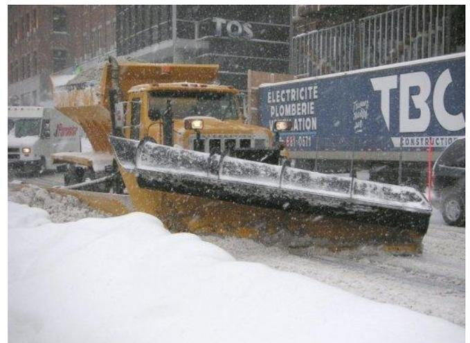
**Fig. 1** All-wheel drive machine for snow removal.
