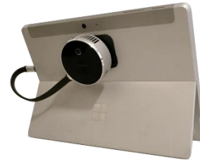
Fig.11 Display of LiDAR sensor and smartphone before scanning [11]
