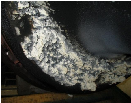
Fig. 5: Contamination by mixing with unburnt oil, carbon, water.
