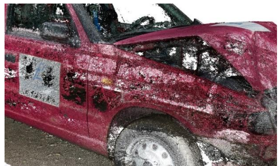
Fig. 7 Building dense points in Agisoft Metashape
