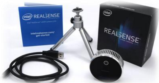
Fig.11 LIDAR camera (RealSence L515) [10]
