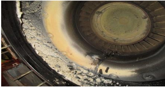
Fig. 4: Presence of unburnt oil along with carbon deposits.
