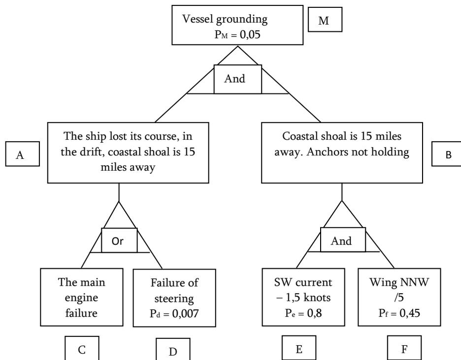
Fig. 3. The fault tree – ES developments (vessel grounding)
