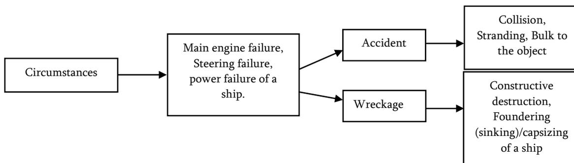
Fig.1. A generalized scheme of scenario for the development of an emergency situation
