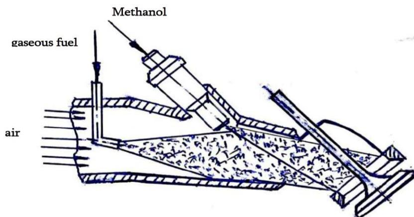
Fig.1. Scheme of the formation of gas-methanol or hydrogen-methanol working mixture
