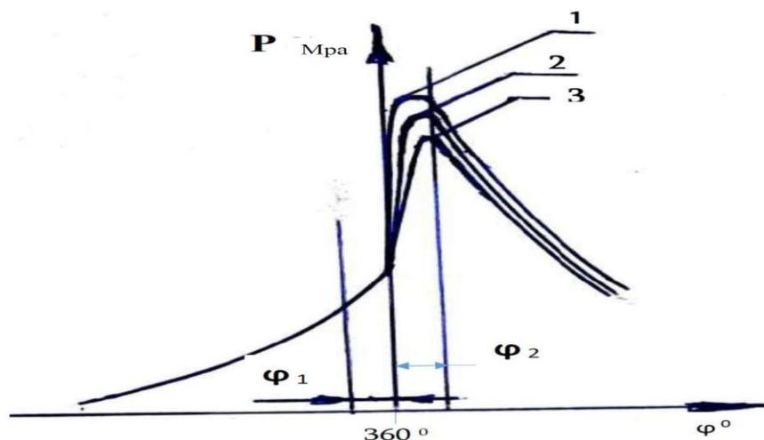
Fig. 2. The theoretical indicator diagram: 1-Hydrogen-liquid gas fuel mixture; 2- Natural gas-methanol fuel mixture; 3- Natural gas fuel mixture.
