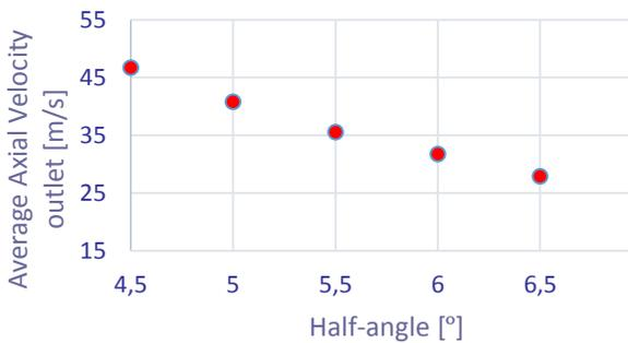
Fig. 9 Dependence of average axial velocity on the outlet on the half angle
