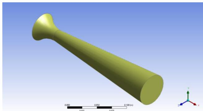
Fig. 5 3D model fluidnog domena restrictora
