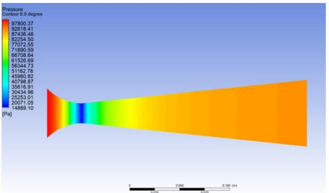
Fig. 13 Pressure contour for half-angle of divergent part 6.0°
