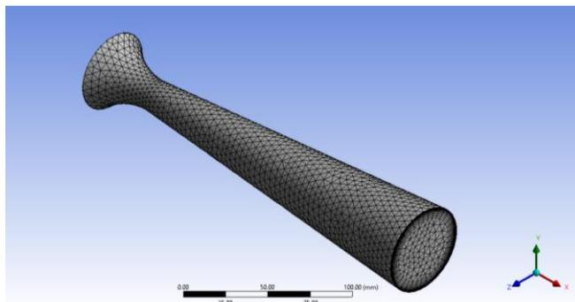
Fig. 6 Mash of fluid domain restrictor
