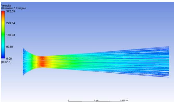
Fig. 17 Velocity streamline for half-angle of divergent part 5.0°
