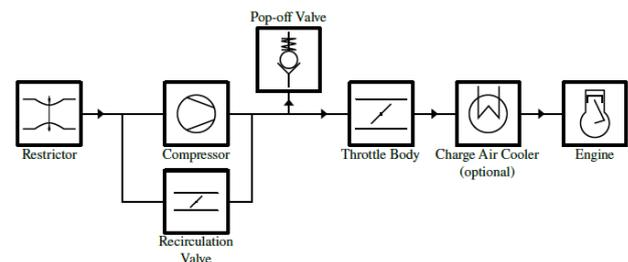
Fig. 2 Configuration for turbocharged or supercharged engines [18]
