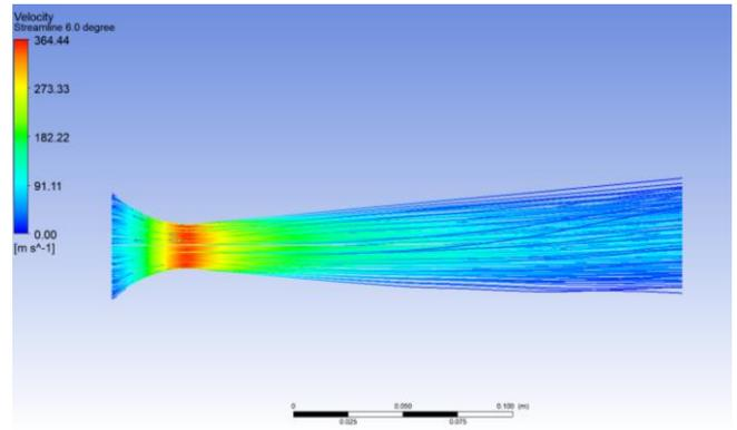
Fig. 19 Velocity streamline for half-angle of divergent part 6.0°
