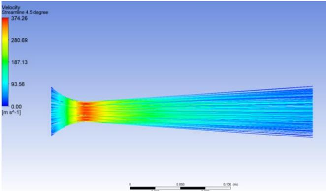
Fig. 16 Velocity streamline for half-angle of divergent part 4.5°
