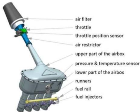
Fig. 3 Design of the assembly of the intake manifold [10]
