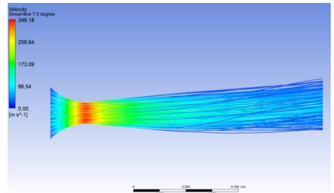
Fig. 21 Velocity streamline for half-angle of divergent part 7.0°
