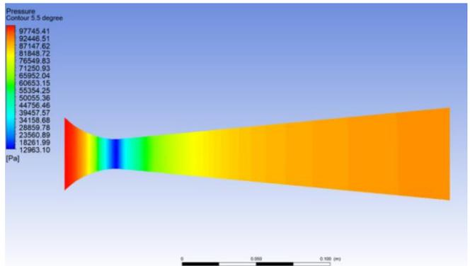
Fig. 12 Pressure contour for half-angle of divergent part 5.5°
