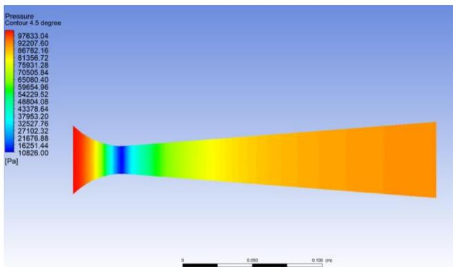
Fig. 10 Pressure contour for half-angle of divergent part 4.5°
