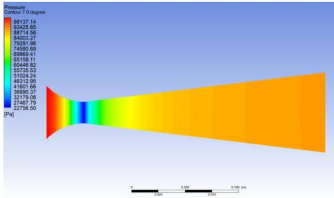
Fig. 15 Pressure contour for half-angle of divergent part 7.0°
