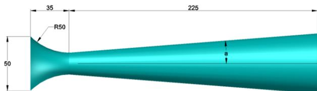
Fig. 4 Dimension of restrictor
