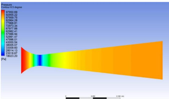
Fig. 14 Pressure contour for half-angle of divergent part 6.5°
