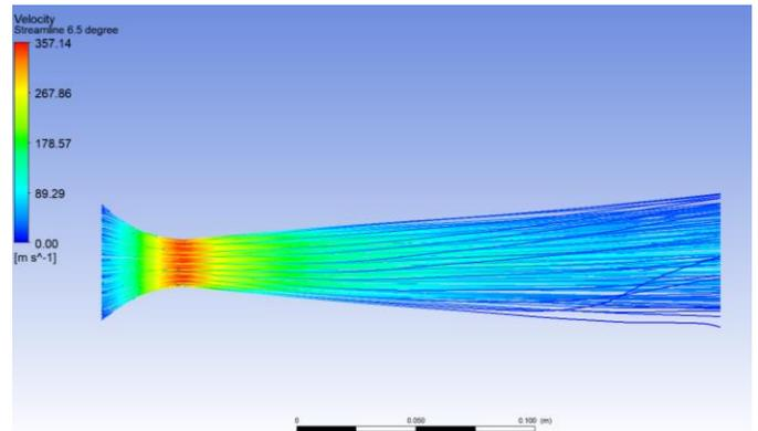
Fig. 20 Velocity streamline for half-angle of divergent part 6.5°
