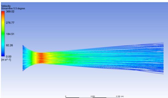
Fig. 18 Velocity streamline for half-angle of divergent part 5.5°
