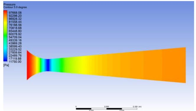
Fig. 11 Pressure contour for half-angle of divergent part 5.0°
