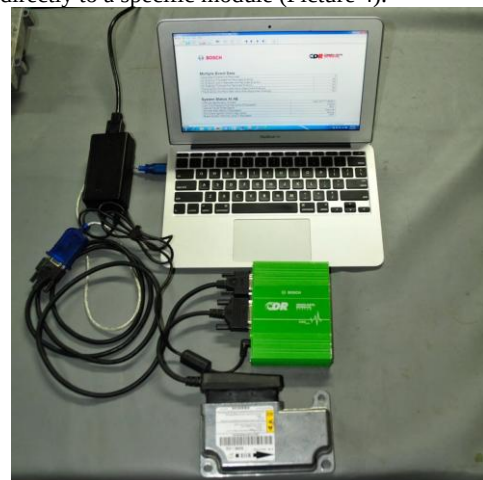
Picture 4. Collecting data from the Event Data Recorder using the "Direct to module" method
