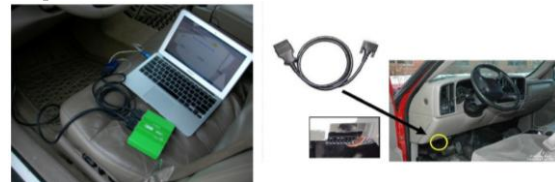
Picture 3. Collecting data with the "Direct to Link" method
