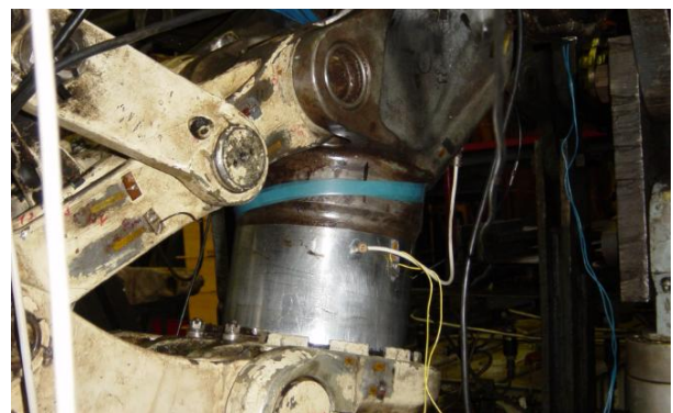
Fig.3 AE monitoring of the shock absorber strut of the main landing gear of the aircraft
