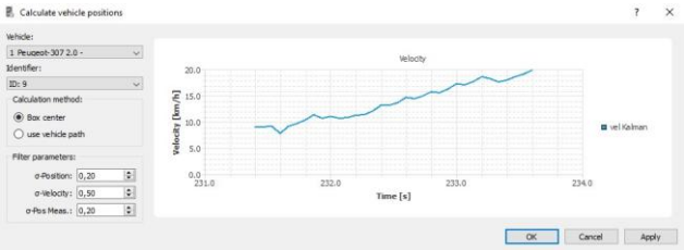
Fig. 15 Vehicle speed diagram determined by video analysis in PC-Crash software
