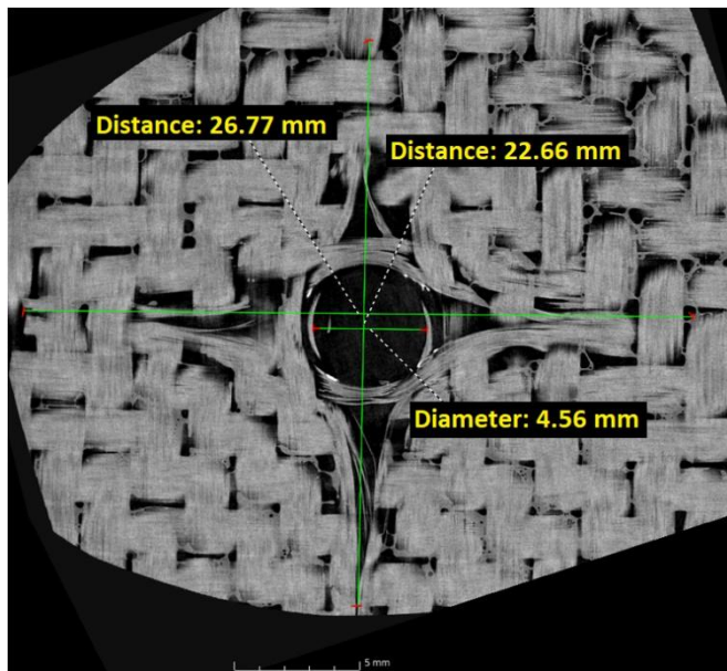
Fig. 5 Fibre distribution around the opening in the CF composite
