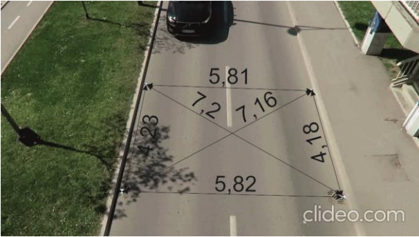
Fig. 1 Layout of the road section on which the analysis was performed with characteristic points and their mutual distances
