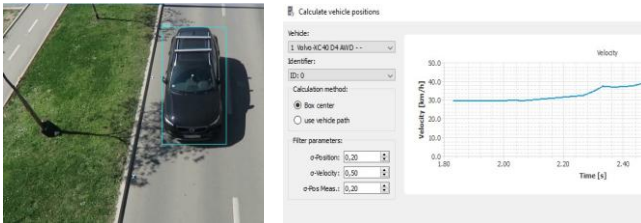
Fig. 6, 7 Identification of the vehicle that was the subject of the investigation, with a speed diagram
