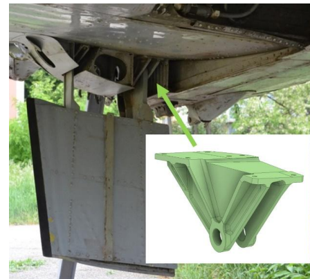
Fig. 1 Air brake bracket location on jet airplane and bracket CAD model.
