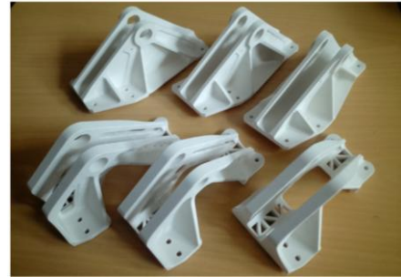
Fig. 8 Experimental brackets made from ASA material.
