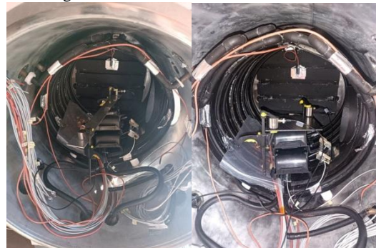
Fig.6. Test specimens (duralumin - left, composite - right) with mounted sensors inside the space environment simulator
